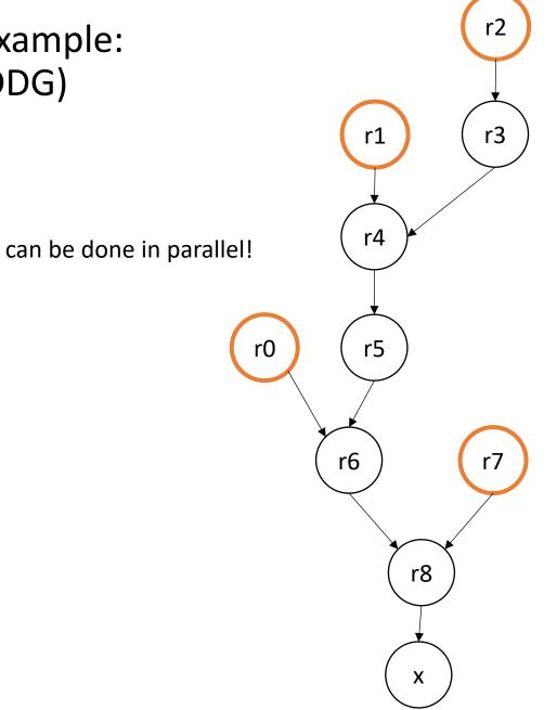
r0 = neq(b);r1 = b \* b; r2 = 4 \* a; r3 = r2 \* c;should we hoist this one? r4 = r1 - r3;r5 = sqrt(r4);r6 = r0 - r5;r7 = 2 \* a;r8 = r6 / r7; x = r8;
