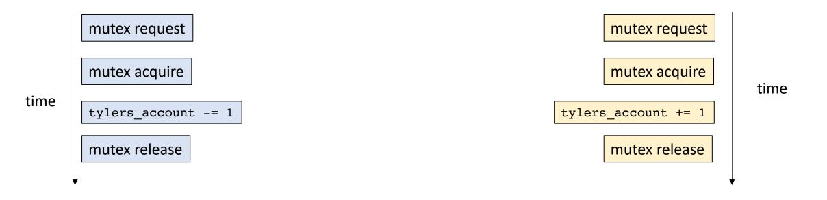
at this point, thread 0 holds the mutex. another thread cannot acquire the mutex until thread 0 releases the mutex also called the **critical section.**
